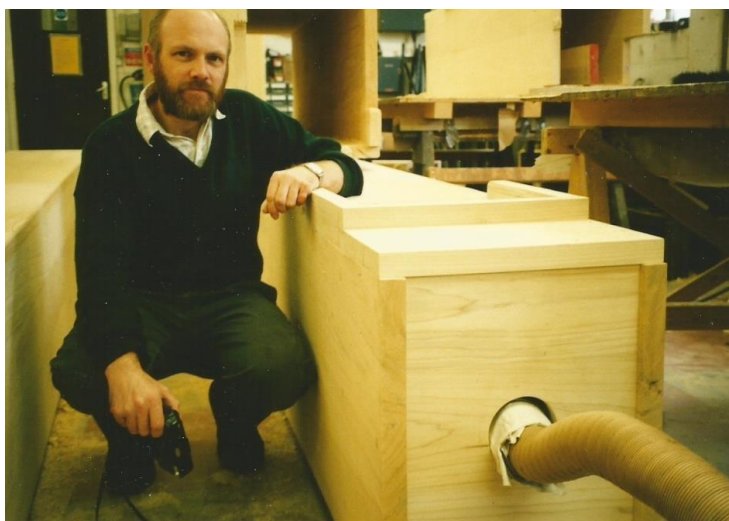
Andrew Pennells at J. W. Walker's works with one of the new 32 foot pipes
